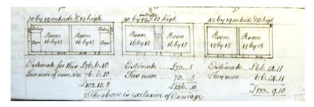
Above I give you three rough Sketches of Plans for Housing at Langley Mill for Smelters etc. upon which I should be glad to have your Opinion. The first 50 by 19 feet Outside and 13 high is upon an Idea that the Persons living in them are to have Cows & the whole Apartmts. for each Family in this way will be
